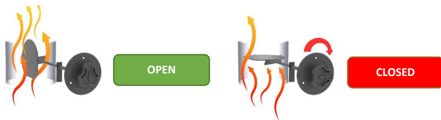
Scheme 3 – Chimney flat regulation
